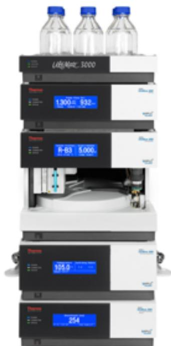
**Figure 2.** An example of an UHPLC system.
